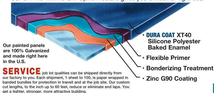
**DURABILITY** Constructed of 29 gauge high tensile steel (to ASTM A792 Grade E, 80,000 minimum yield), our G90 ribbed panels are easy to install, sturdy and weather tight. Resistance to dents, plus minimal expansion/contraction properties make this steel panel an excellent investment providing lasting protection and greater durability that will enhance all types of structural designs.
